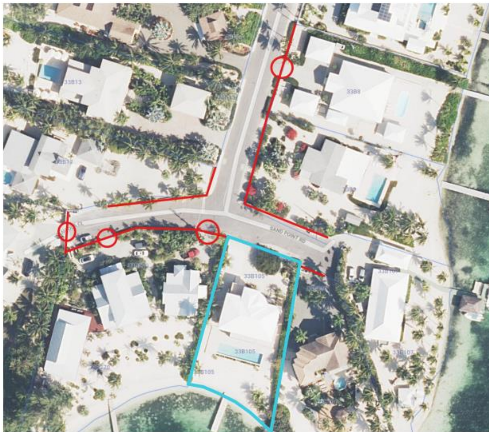
Fig. 5. Red lines represent existing roadside boundary walls with zero setbacks.
