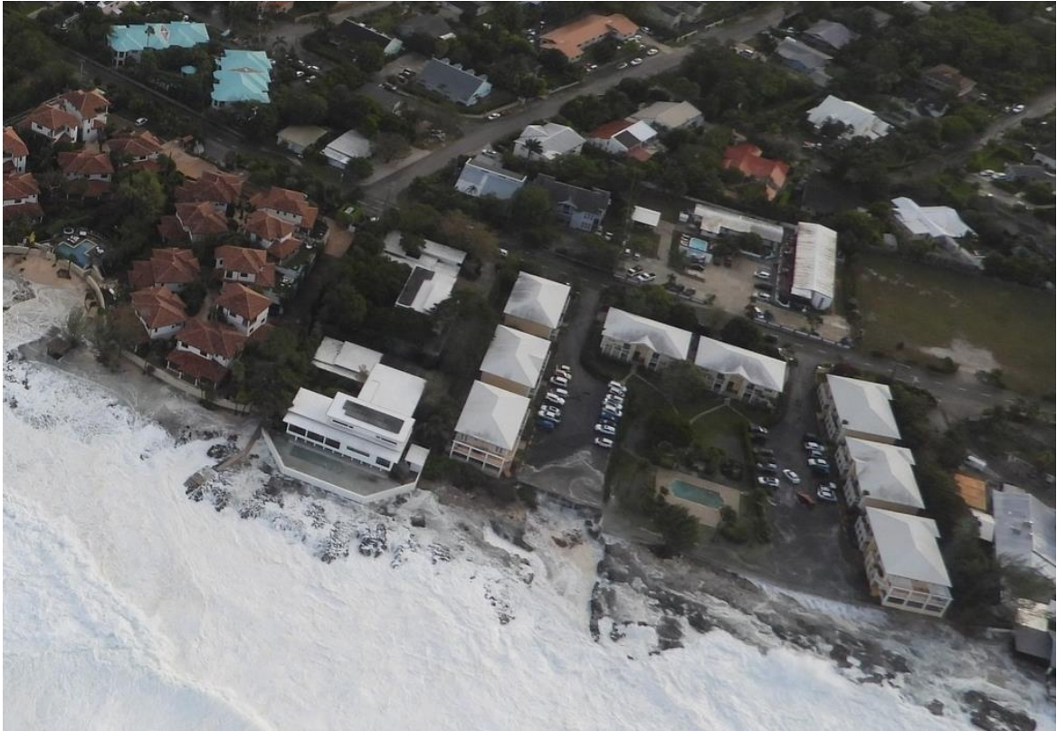
Figure 3. Aerial imagery from the Nor'wester of February 2024 showing the waves overtopping the seawall at a nearby development. The existence of a man-made cut in the ironshore has brought the waves further into the development. (Aerial Imagery Source: RCIPS, 2024).
