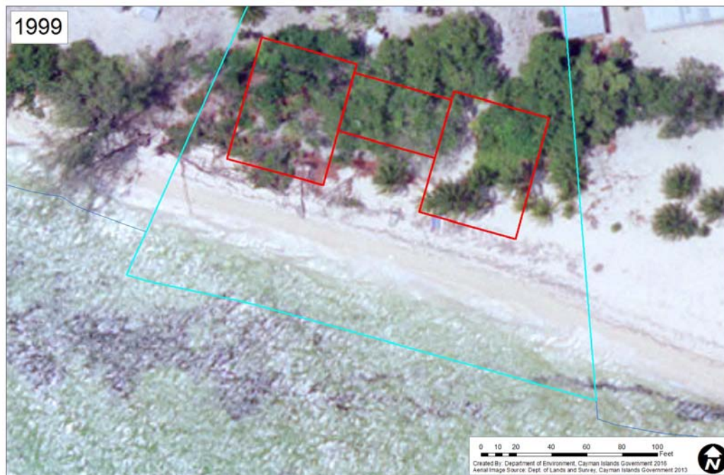
Figure 3: 1999 aerial image with the current registered boundary and the proposed building footprint overlaid to show HWM variation (LIS 1999)
