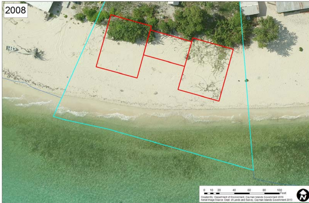
Figure 2: 2008 aerial image with the current registered boundary and the proposed building footprint overlaid to show HWM variation (LIS 2008)
