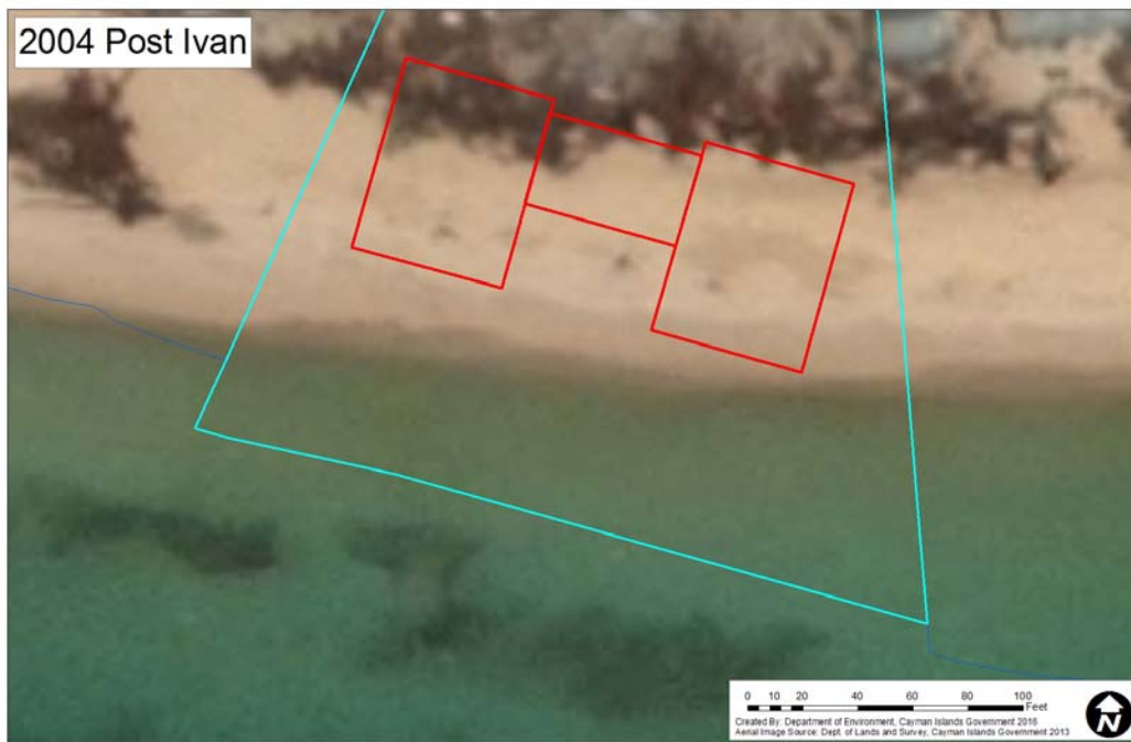
Figure 3: 2004 post hurricane Ivan aerial image with the current registered boundary and the proposed building footprint overlaid to show HWM variation (LIS 2004)
